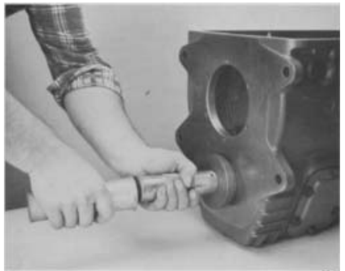
8. If previously removed, install snap ring, countershaft front bearing race (from inside of case) and bore plug. Coat outer diameter of bore plug with Loctite #510 before installing.
