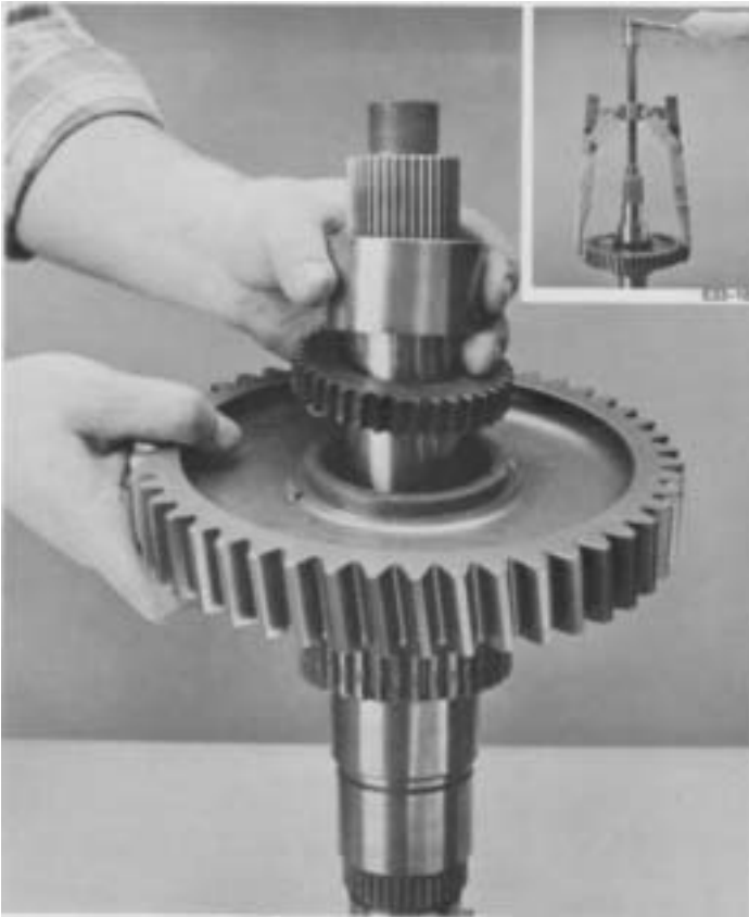
18. Using a puller (inset) or press remove 1st gear, clutch hub, and reverse gear bearing race from mainshaft.
