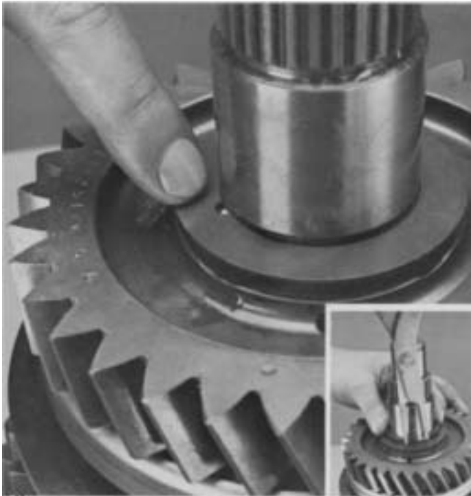
17. Install locating ball and washer. Washer can be installed either way. Install snap ring as shown (inset).
