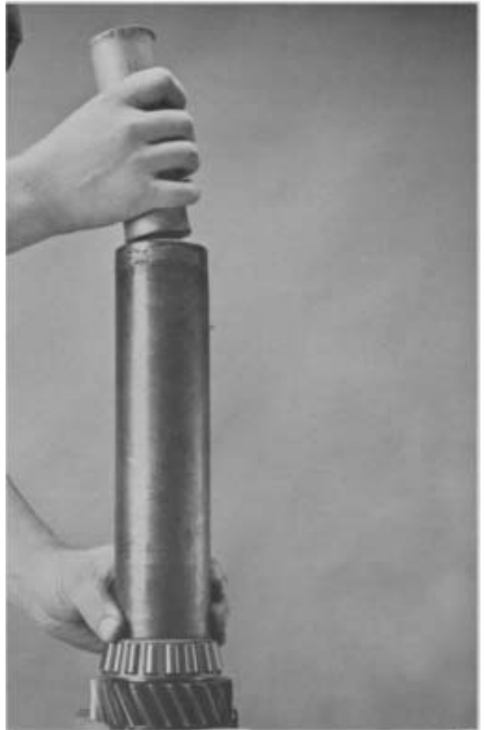
24. Using a sleeve type driver install bearing on input shaft.
