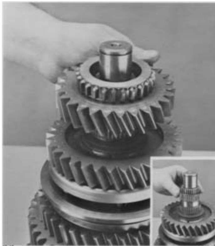
18. Lubricate and install 5th gear bearings (inset). install 5th gear, clutching teeth facing up.
