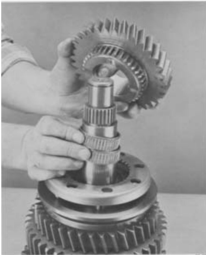
8. Remove 4th gear and bearings.
