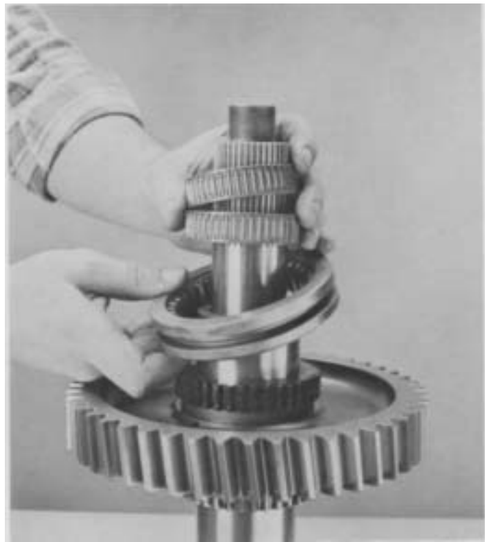
17. Remove reverse gear bearings and reverse gear sliding clutch.
