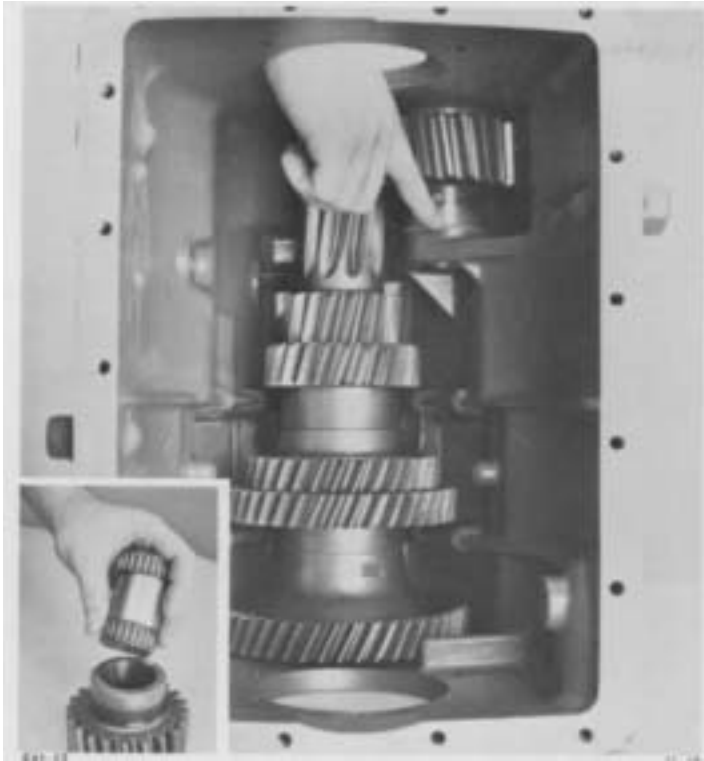
12. Install bearings and spacer in reverse idler gear (inset) and position gear in housing with long hub of gear toward the front.
