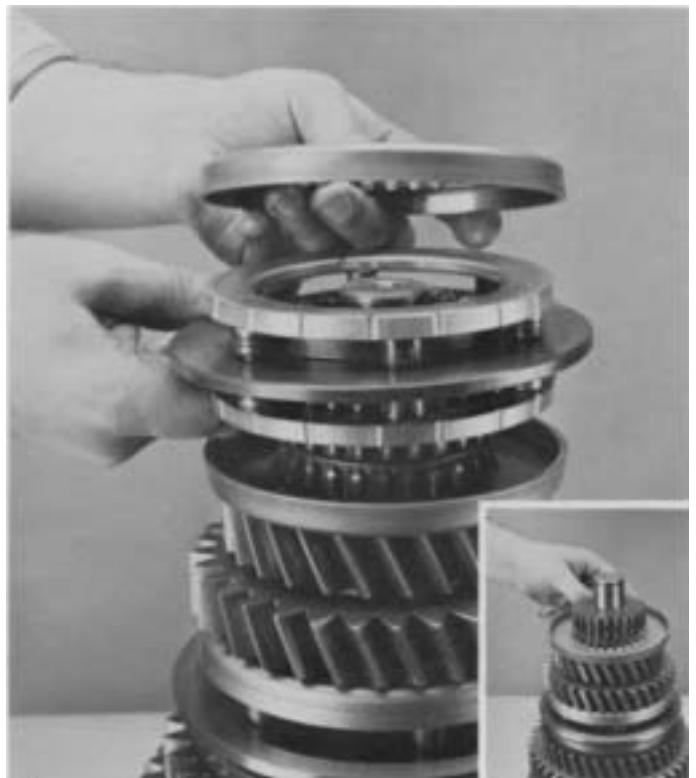
20. Install 5th speed synchronizer cup (inset). Lubricate friction surface with transmission lube and install 5th-6th speed synchronizer assembly and 6th speed synchronizer cup.
