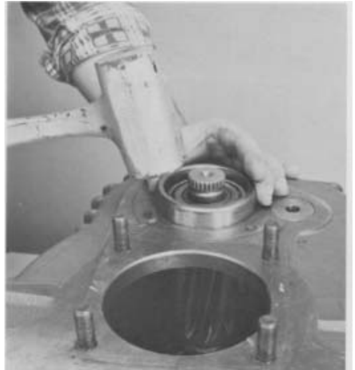
14. Install countershaft rear bearing race into case as shown.
