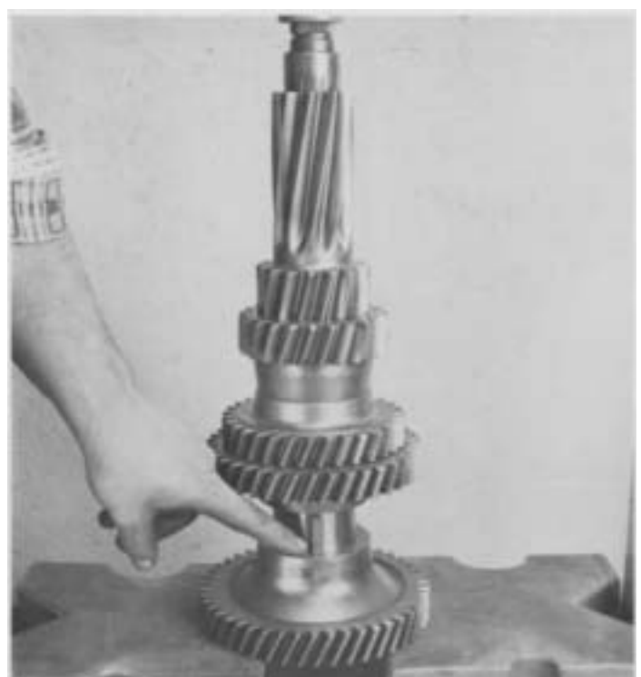
4. Align keyway of drive gear to key on countershaft. Press drive gear on, long hub of gear to rear of shaft.
