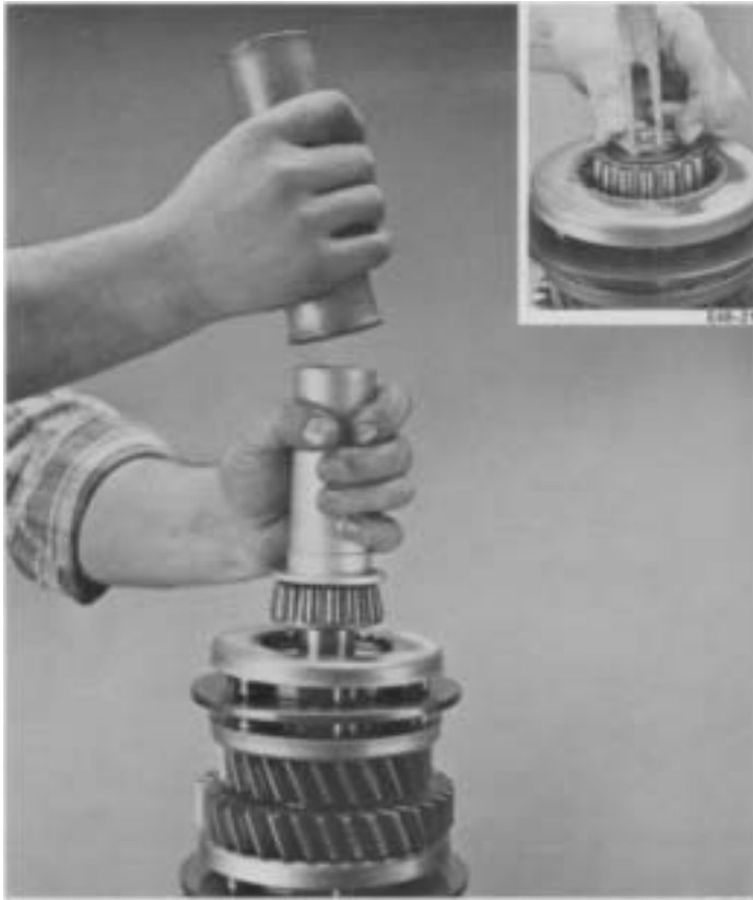
21. Using a sleeve type driver install front mainshaft bearing. Install snap ring in groove on end of shaft (inset).
