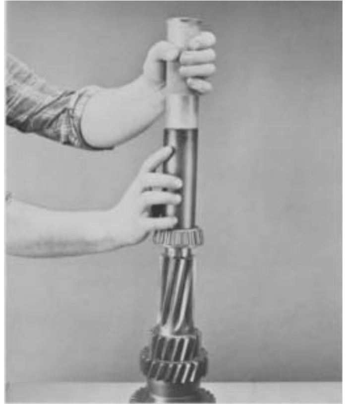
7. Install rear countershaft bearing as shown.
