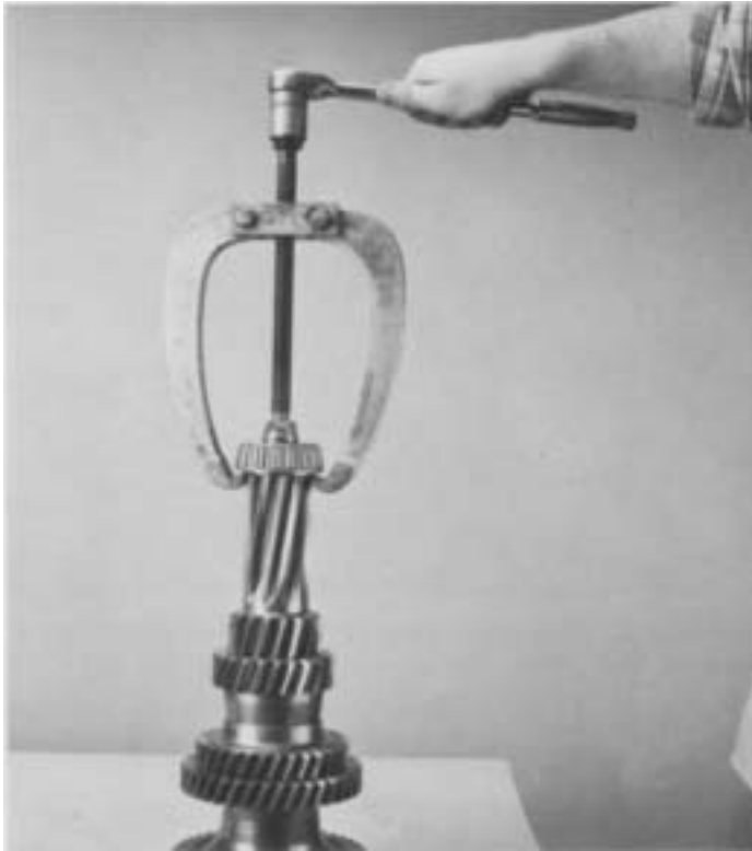
7. Position puller jaws behind rear countershaft bearing and remove bearing.
