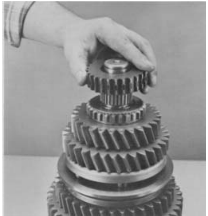
19. Install 5th-6th clutch hub with flat surface facing up.
